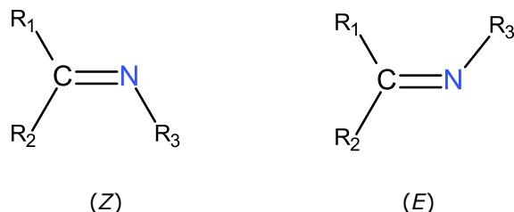
**Slika 1.** Prikaz opće strukture Schiffove baze ( $R_1 = H, \text{alkil, aril}; R_2 \text{ i } R_3 = \text{alkil, aril}$ ).
