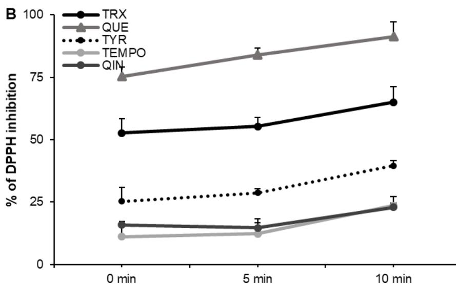
**Figure 47. Antioxidative capacity of A) DA-dopamine, L-DOPA, TYRA-tyramine and B) QUE-quercetin, TYR–tyrosol, TEMPOL and QIN-quinine measured in methanol by DPPH assay.** The results are presented as a percentage of inhibition of the absorbance at 515 nm (absorption max for DPPH) in time points of 0, 5 and 10 minutes for 0.09 mM concentration of all tested molecules. Data are plotted as average of triplicates.
