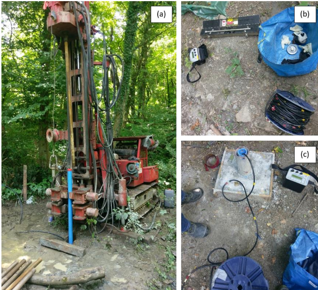
Figure 10: Details of a) inclinometer chasing installation at the B1 location; b) portable inclinometer measuring system Digitilt Classic Inclinometer System (Durham Geo-Enterprises, Inc.); and c) measurements in progress.
